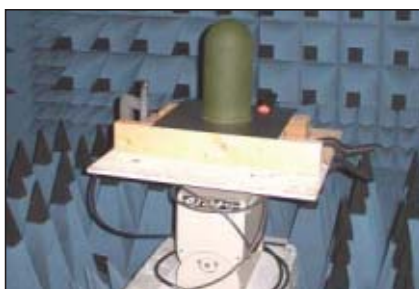
▲ Fig. 10 TASH monopole mounted in the anechoic chamber for azimuth pattern measurements.
